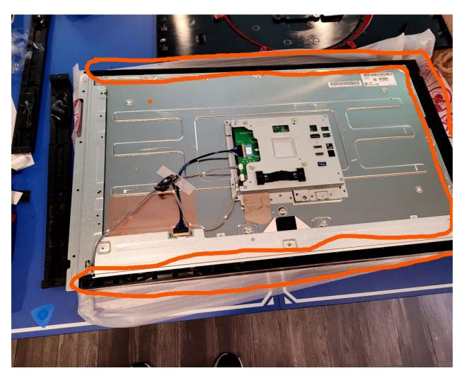
Next you will take one of those metal brackets you removed from the original monitor and place in on one end of the LG monitor sitting in the frame. You will tuck one corner of the bracket under the metal plate on the LG monitor, all while lifting the wire as to not crimp or damage it. See pic below.
